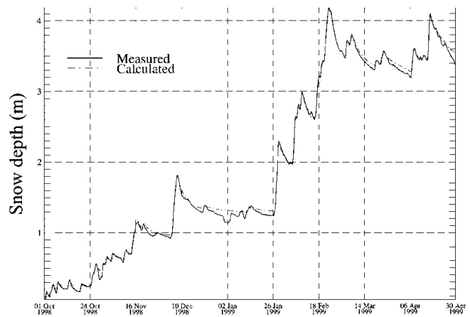
Fig. 1. Comparison between measured and modelled snow depth for the station Klosters. The model is run without the snowdrift routine. The station shows negligible snowdrift influence. Due to measurement errors, the measured curve is always less smooth than the model curve.
