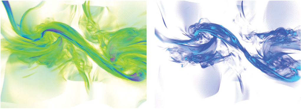
Figure 4. Snapshots of a zoom on the current density (left) [as in Fig. 3 but with a different perspective], and of the enstrophy density \omega^2 (right) at the same time ( t = 4 ) as in Fig. 3 and for the same Taylor-Green (TG) flow with an Iroshnikov-Kraichnan spectrum (see Lee et al. 2010); 2048^3 equivalent grid resolution with a code implementing the symmetries of the TG flow generalized to MHD (see §2). Note the overall spatial correlation between both sets of structures, but with more complexity in the vorticity field.
