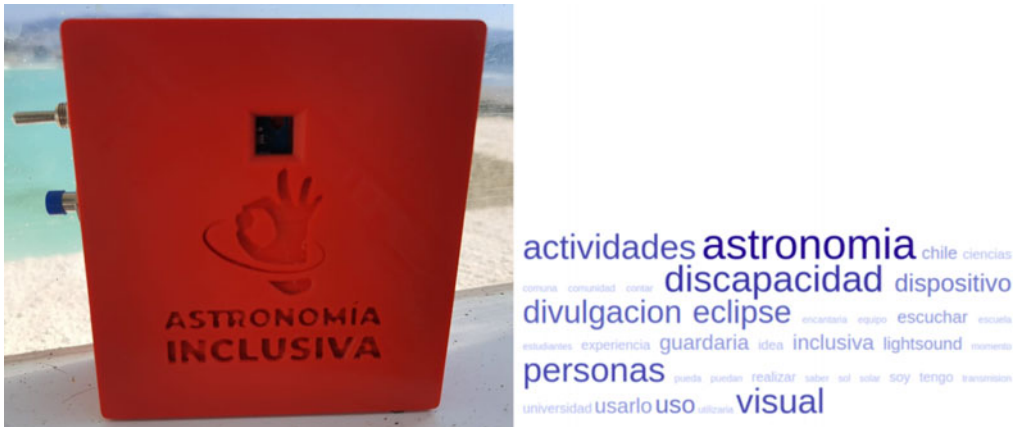
Figure 1. Left: LightSound device for the Eclipse 2020 in Chile. The case was specifically design to adjust all electronic supplies and printed in 3D. In front, the light detector is placed. To the left side, the switch on/off bottom is located, the blue switch change between the tone and musical mode. The logo of our association “Astronomía Inclusiva” is on front of the image. Right: Thirty most used Spanish words in our application form to request a LightSound.
