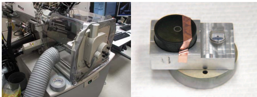
Figure 1 a) Plexiglas enclosure designed to control radiological contamination b) custom met mount and FIB grid holder to enable extraction of samples from highly radioactive fuel samples.
