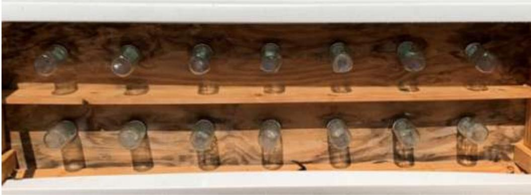
Figure 2. Bottom view of the constructed simulated bed with 14 glass jars attached representing a transplant crop hole. Top row are jars 1-7 (left side of bed) and the bottom row are jars 8-14 (right side of jars), with jars being opposite going down the length of the bed (i.e., jars 1 and 8 are across from each other, etc.). Holes were spaced 30.5 cm apart from the center of one hole to the center of another and 20.3 cm from the center of one hole to the edge of the plywood
