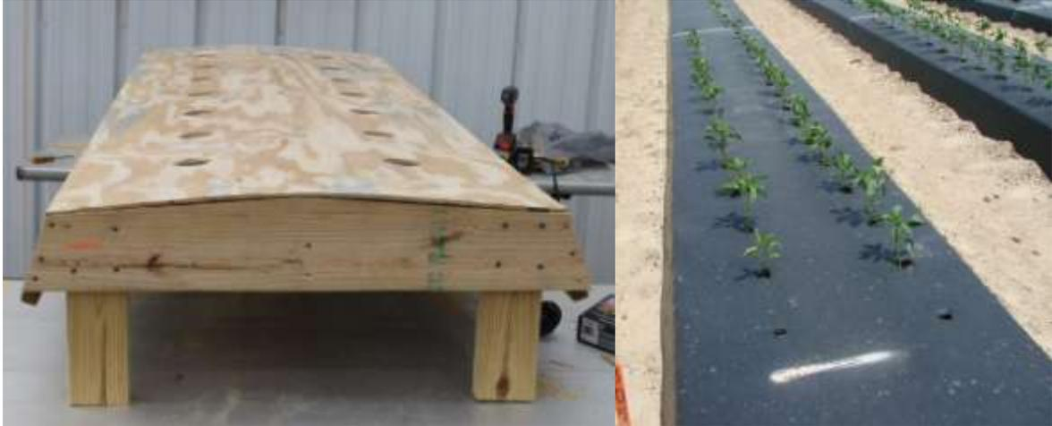
Figure 1. Bed construction without carpet or plastic mulch covering. Design of the simulated bed was created to mimic a soil bed used in pepper production, including a slope of 6.7% from the middle to each side of the bed, in comparison to an actual field bed.
