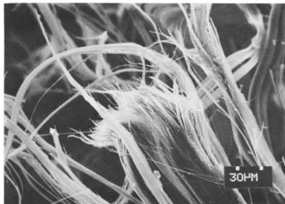
Figure 3. Scanning electron micrograph of woolly erionite from a joint in mudstone, Reese River, Nevada.
