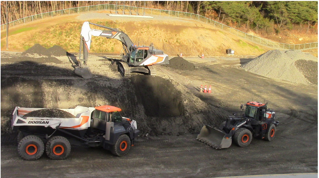
Figure 7. Teaming of autonomous machines in Concept-X [43].
