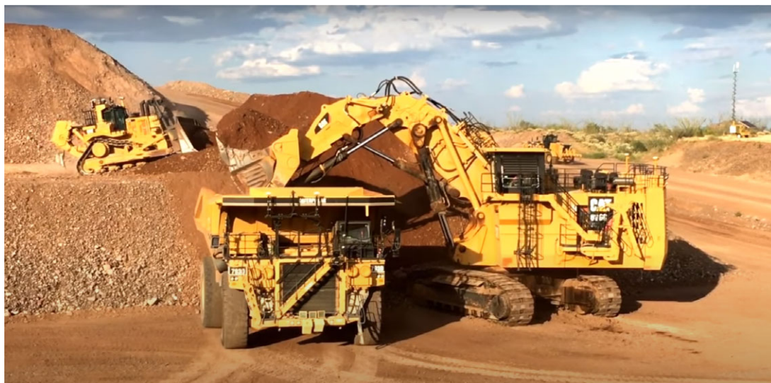
Figure 4. Caterpillar autonomous equipment teaming on a surface mine [82].
