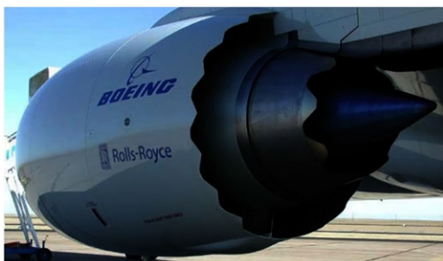
Figure 6. Serrated nozzles on both by-pass and core ducts on Boeing 787 aircraft.
