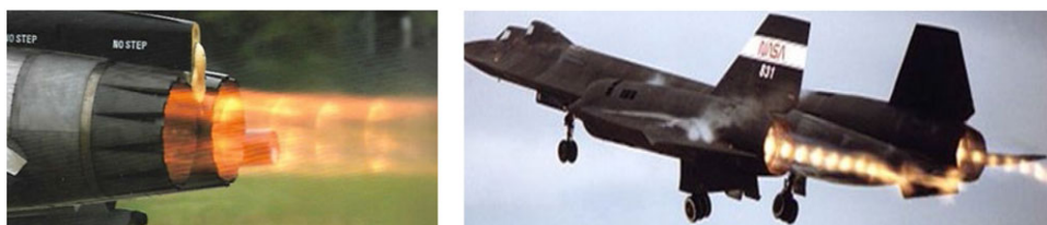
Figure 8. Examples of shock-containing hot jet plumes.
