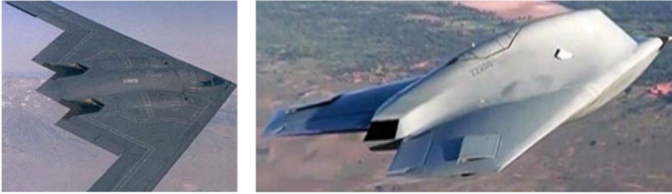
Figure 9. Non-axisymmetric nozzle cross-section with aft-deck: B2 (left) and BAeS-Taranis (right).
