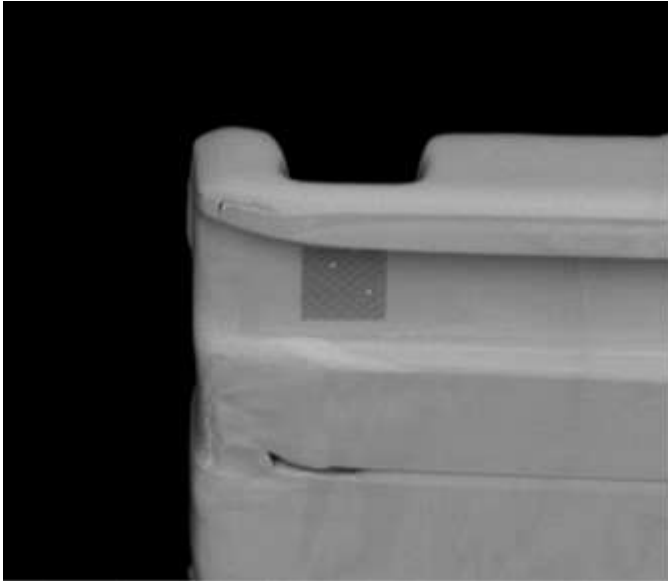
Figure 2. Figure 2: This figure shows a SEM image taken from the first side of a completed BEOL plan view TEM sample prepared using the crossing FIB box method.
