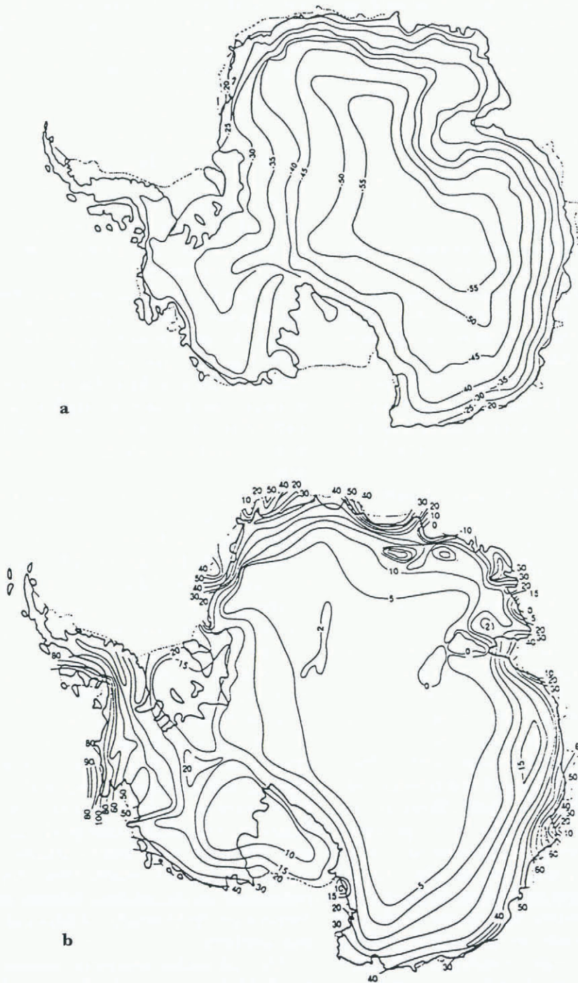
Fig. 2. (a) Mean annual ice-sheet surface temperature ( ^{\circ}\text{C} ), based on surface measurements of Antarctica. Adapted from Robin (1983). (b) Mean annual surface mass-balance distribution on Antarctica. Values are in water equivalent \text{cm year}^{-1} . Adapted from Giovinetto and Bentley (1985).
