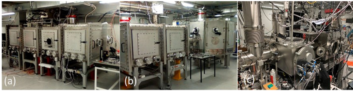
Figure 24. The SCAPA laser facility interaction areas: (a) Beamline A2 in Bunker A; (b) Beamline B2 in Bunker B; and (c) work in progress on the ALPHA-X/medical beamline in Bunker C.
