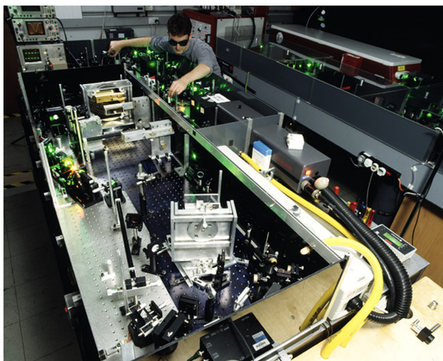
Figure 8. Imperial College's terawatt 150 fs, 150 mJ Ti:sapphire CPA system circa 2000 being adjusted by the then PhD student Mike Mason. (Picture courtesy of Imperial College London.)
