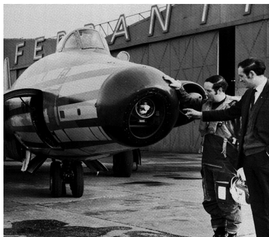
Figure 74. Reviewing the installation of the prototype LRMTS onto the Canberra test bed at Turnhouse Airport circa March 1971. (Picture courtesy of Leonardo.)
