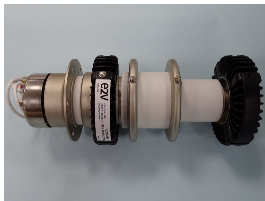
Figure 65. EEV's CX1625A hollow anode thyatron designed for excimer lasers.
