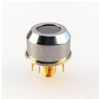
Figure 1. Detector module with metal cap and 1 μm graphenic window.
