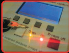
Packaged tubes come with integral high voltage power supplies and may be operated up to 50kV. Power supplies are integrated with interlocking vacuum sensors that shut off x-rays when the SEM chamber is vented. Every unit automatically “ramps” the tubes for increased longevity.
