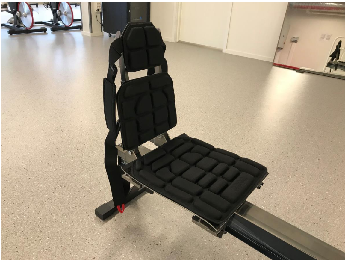
Figure 2. Rowing ergometer adapted for PR1 Paralympic rowers by installing a fixed seat
