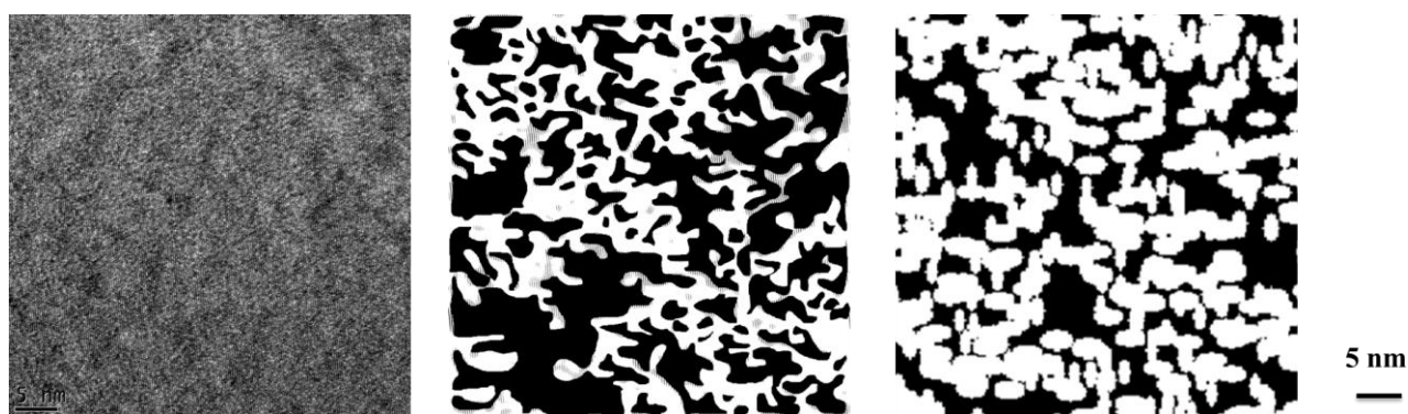
Figure 1. (a) HRTEM image of SiC irradiated up to 50% of the dose to amorphization at Mag=470 kx. (b) Fourier filtered image. (c) Simulated images. (In (b) and (c), black represents crystalline and white represents amorphous.)
