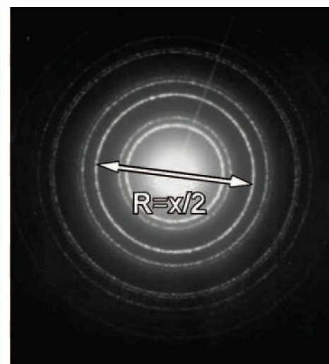
Fig. 4: Electron diffraction pattern from an unknown sample, suspected to be aluminum.
