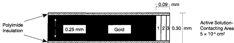
A cross-section of the subcutaneous microsenor described by Adam Heller of the University of Texas-Austin in his Symposium X talk on Electron Conducting Redox Hydrogels. Such microsenors could be implanted in humans to monitor glucose levels in diabetics. The sensing layer 1 is covered by a dynamic range expanding layer 2 and a biocompatible layer 3. The overall diameter is 0.3 mm.
