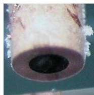
Figure 1: Image of the crosssection of copper tube filled with ice. White spot near the center is an area with crystalline ice.
