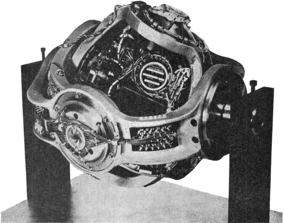
*Fig. 1. Miniature platform for inertial guidance.*
