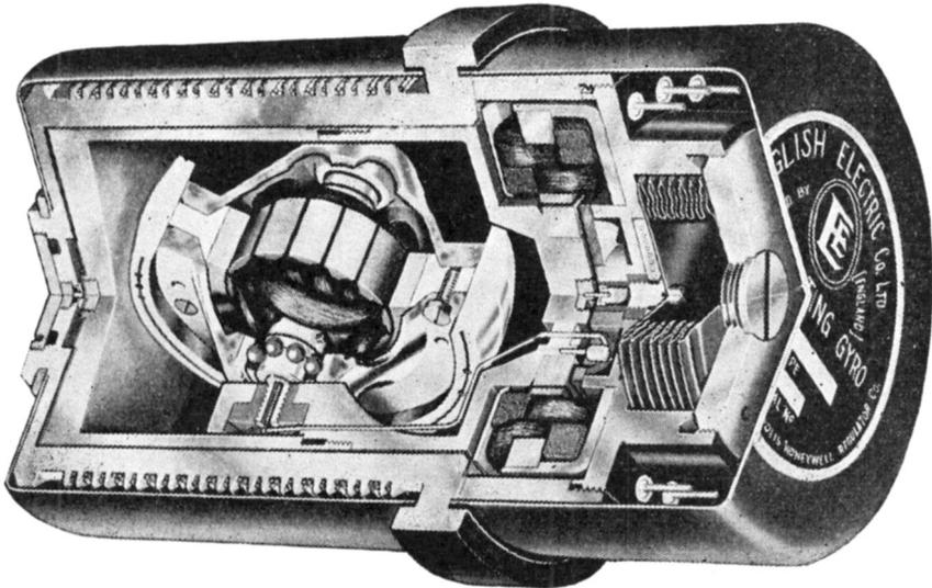
*Fig. 3. Miniature rate-integrating gyroscope.*
