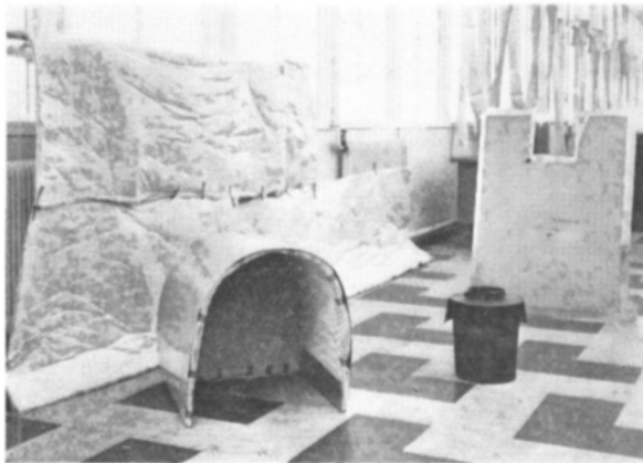
Fig 12 Sound absorbent head shield (2 ft × 2 ft × 2 ft) and other components used in Whirlwind cabin noise tests
