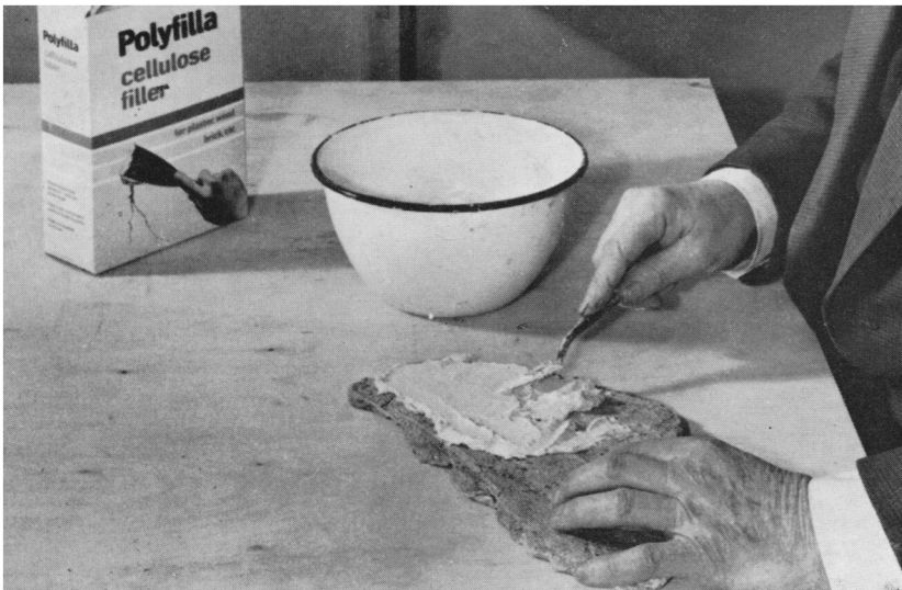
B. Wall-plaster reversed and reinforced with scrim and adhesive (p. 258).
