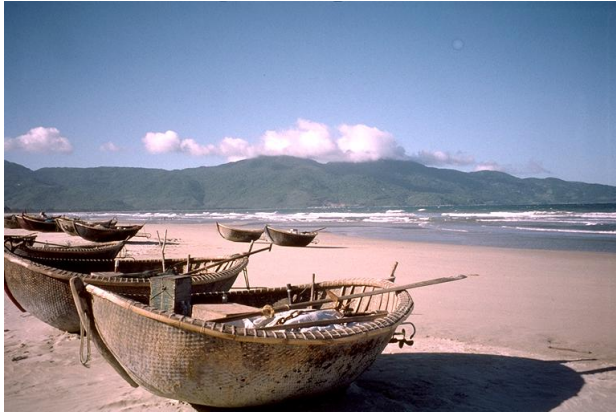
Bamboo basket boats, Vietnam, 2000. Traditionally caulked with resin and fillers such as sawdust, shredded bamboo or cattle dung. Courtesy University of Hawai'i Center for Southeast Asian Studies picture archive
