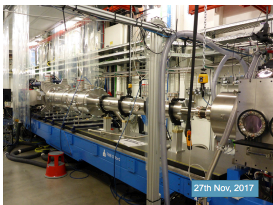
Figure 1. Photograph of the SPB/SFX instrument of the European XFEL set up in “long” (~5.5 m) sample to detector geometry for single particle imaging of ~ 500 nm diameter samples.
