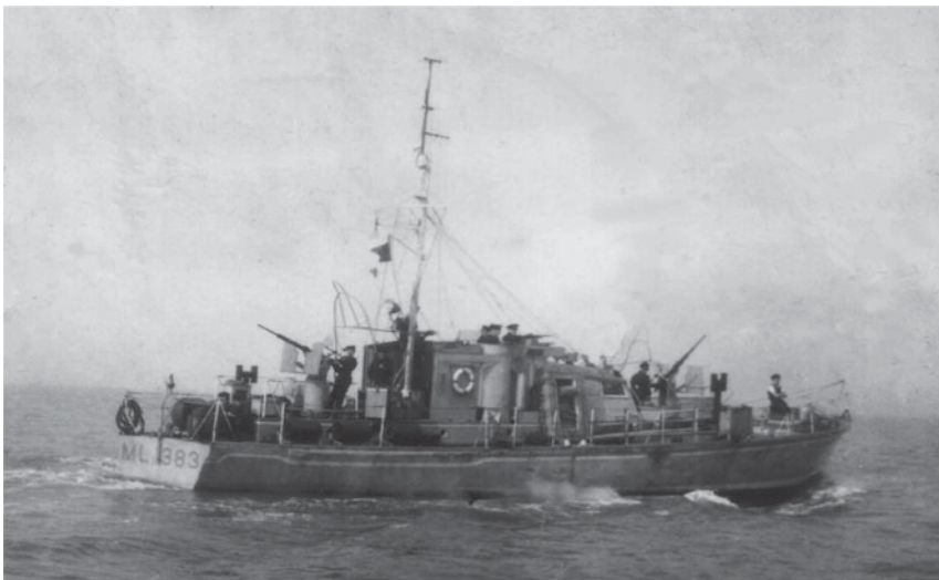
Figure 10. HDML 1383: Decca aerial was a wire strung up to the mainmast.
