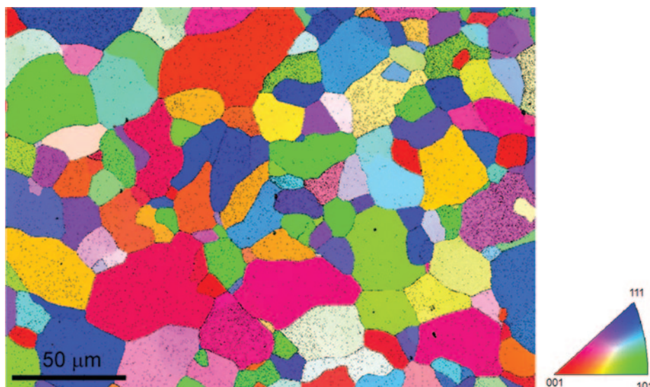
Figure 2: High-quality EBSD inverse pole figure map of a magnetic alloy (raw data). There were 585,000 patterns collected for this image with 95.7% successfully indexed. Note that many of the unindexed pixels were at grain boundaries or at second phase inclusions (black). The color key for the image (stereographic triangle) is shown at right.
