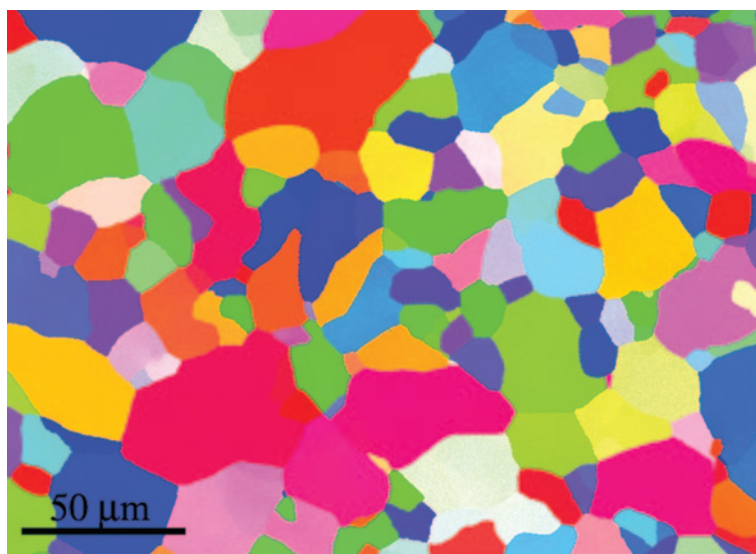
Figure 3: The same map as in Figure 2 with the misindexed and unindexed pixels removed, using a 6-neighbor rule, iterated 6 times. Note that none of the second phase inclusions are represented in the microstructure.
