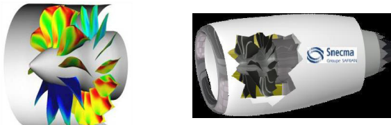
Counter rotating fan with 10 + 14 blades
