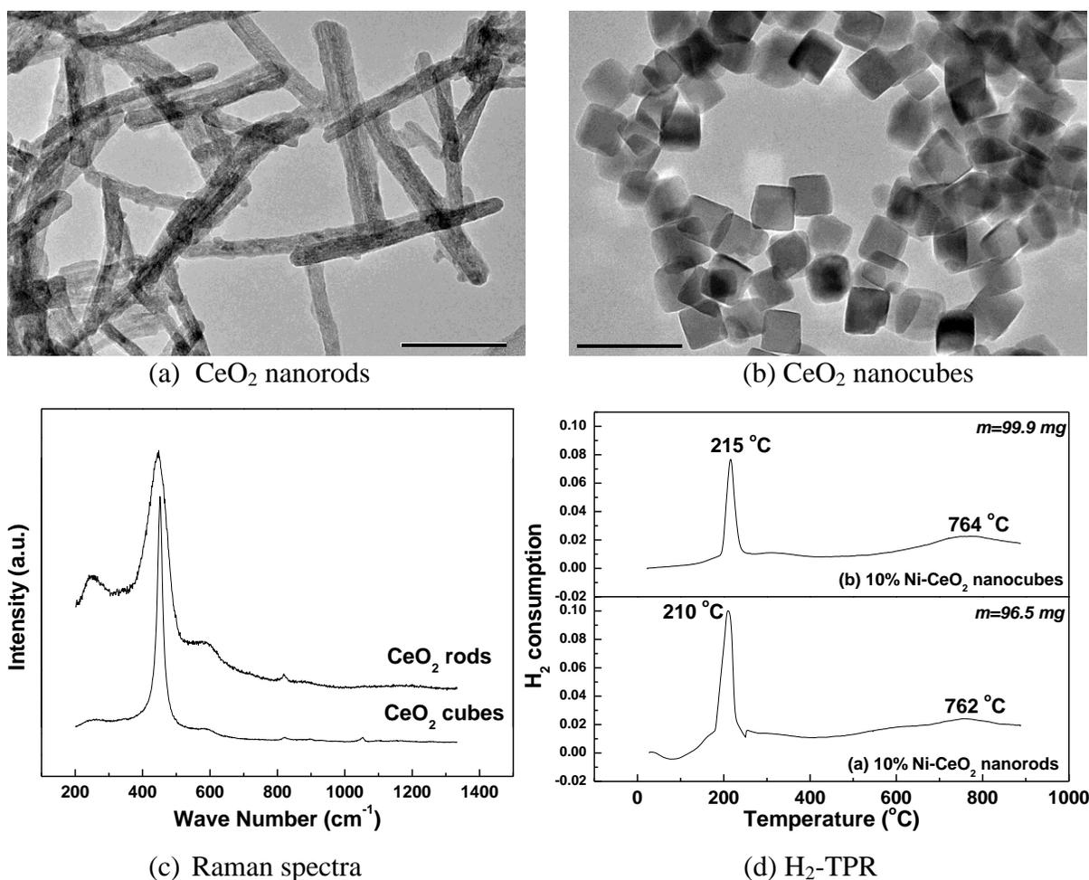
Figure 1 TEM images (a)/(b) (scale bar: 50 nm) and Raman spectra (c) of CeO<sub>2</sub> nanorods and nanocubes, and H<sub>2</sub>-TPR profiles (d) of 10wt% Ni/CeO<sub>2</sub> nanorods and nanocubes under a 5% H<sub>2</sub>/95% Ar gas atmosphere.
