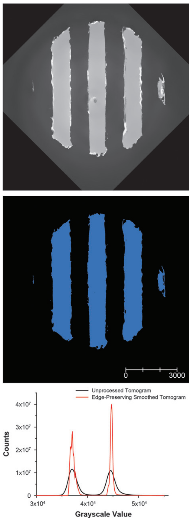
Figure 5: Top: The same slice as presented in Figure 2A (top left), after applying an edge-preserving smoothing filter. After the smoothing step, the tomogram was segmented (middle) for the foam material. The scale bar is in micrometers. Bottom: The grayscale histograms of the tomograms before and after applying the edge-preserving smoothing filter.
