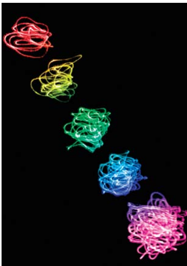
Plasma emission from collapsing bubbles: The imploding bubbles move around after each collapse, tracing out a lit path, like a person flinging their arm around while holding a flashlight. Photo courtesy Hangxun Xu and Ken Suslick.
