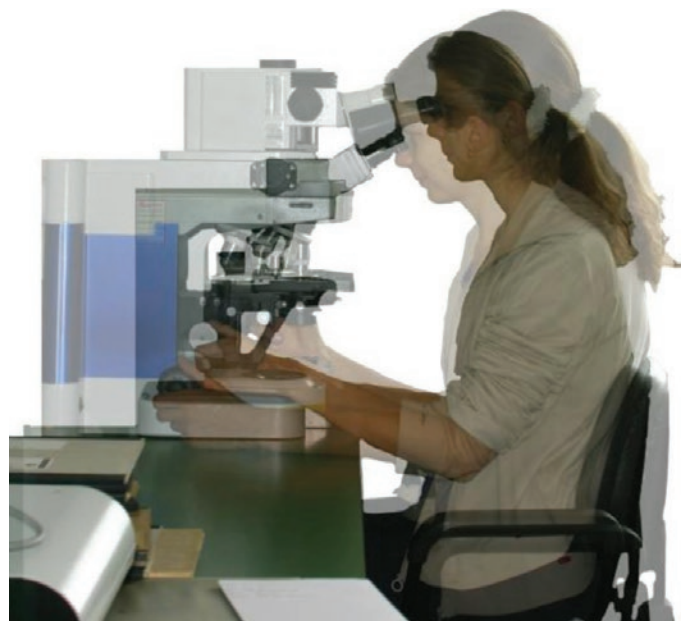
Figure 3: Comparison of traditional and modified microscopes. Existing (old) microscope and tube (background image) and Axio Imager with Ergotube 50-15-50 (foreground image).
