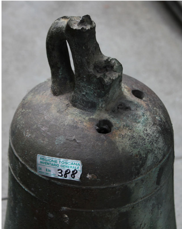
Fig 13. Broken crown and holes on the top part of bell no 8. Image: Attilio Tori, with permission.
