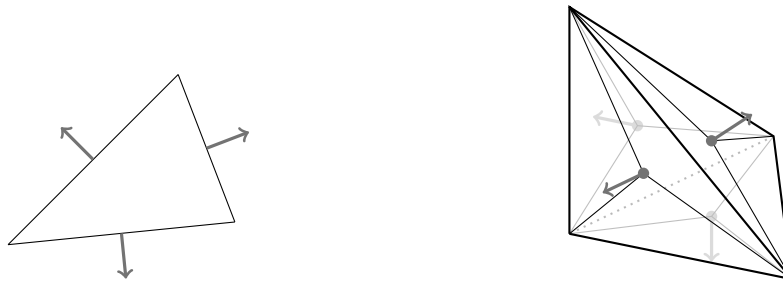
Figure 5: The Raviart-Thomas functions in \mathbb{R}^2 and \mathbb{R}^3 of the form v(x_1, x_2) = (a_1 + b x_1, a_2 + b x_2) , have three resp. four degrees of freedom. For each face, the normal component can be chosen - the resulting functions are H(\text{div}) -conforming.
