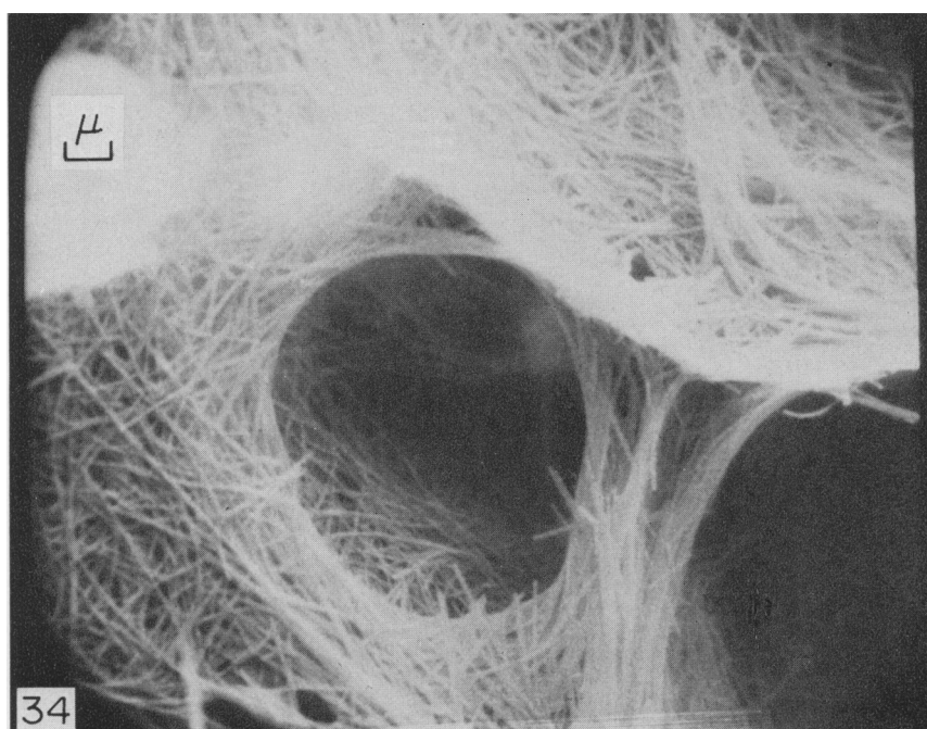
Fig. 33. Scanning electron micrograph of intertwined mordenite fibers with clinoptilolite from an ash-flow tuff near Monolith, California. This tuff has been mined by Monolith Portland Cement Company as a pozzolan. (Sample 25-5-5)
