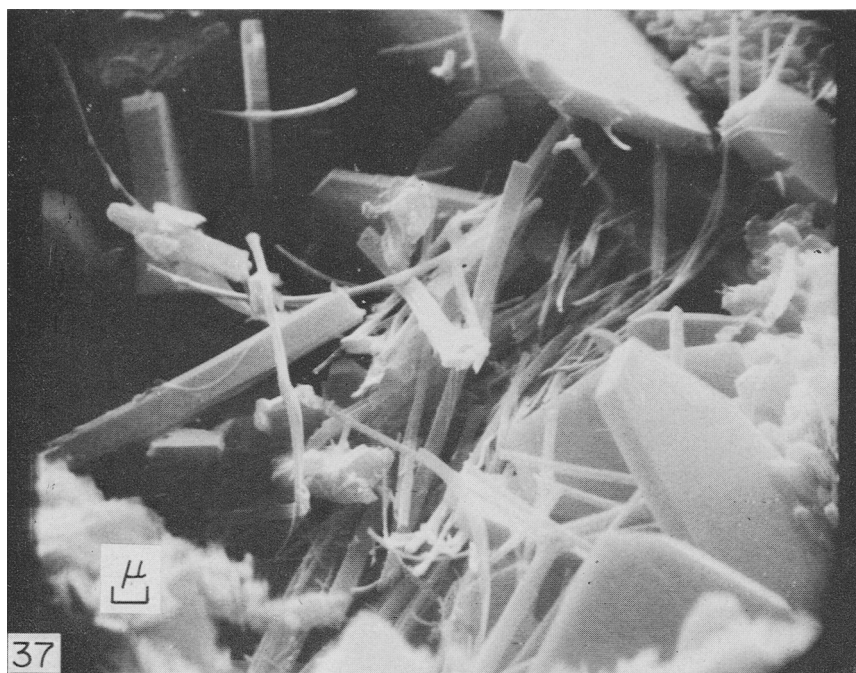
Fig. 37. Scanning electron micrograph of needles and fibers associated with clinoptilolite from a marine tuff near Dzegvi, Georgia, U.S.S.R. Although erionite or mordenite is suspected, neither can be identified from morphology alone, nor has either been detected in the sample by X-ray diffraction examination. (Sample 25-23-6)
