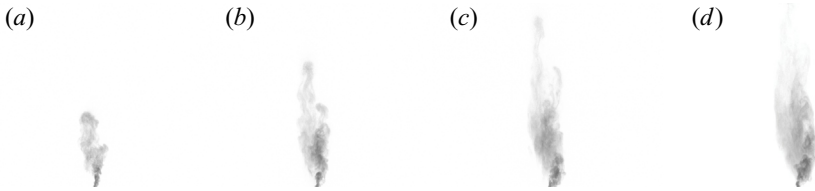
Figure 15. Illustration of rising plume fingers for series C and Ro \approx 0.048 ( \Omega = 1 \text{ rad s}^{-1} ) for four consecutive times. The plume fingers appear to be stretched and to become thinner as the time progresses: (a) \Omega t \approx 2\pi ; (b) \Omega t \approx 4\pi ; (c) \Omega t \approx 6\pi ; and (d) \Omega t \approx 8\pi .
