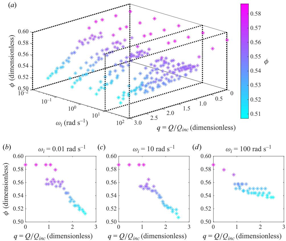
Figure 3. Measurements of the solid fraction  $\phi$  as a function of normalized fluidization rate  $q$  and rotational speed  $\omega_i$  for *FBI* with mean diameter  $D = 113 \mu\text{m}$ . At  $\omega_i = 0$ , intermittent bubbling can be seen within the bed volume starting at  $q = 1.1$ . Beyond this flow rate, the estimated volumetric solid fraction,  $\phi$ , decreases with respect to  $q$ , as found for  $\omega_i = 0.01, 10$  and  $100 \text{ rad s}^{-1}$  in (b), (c) and (d).
