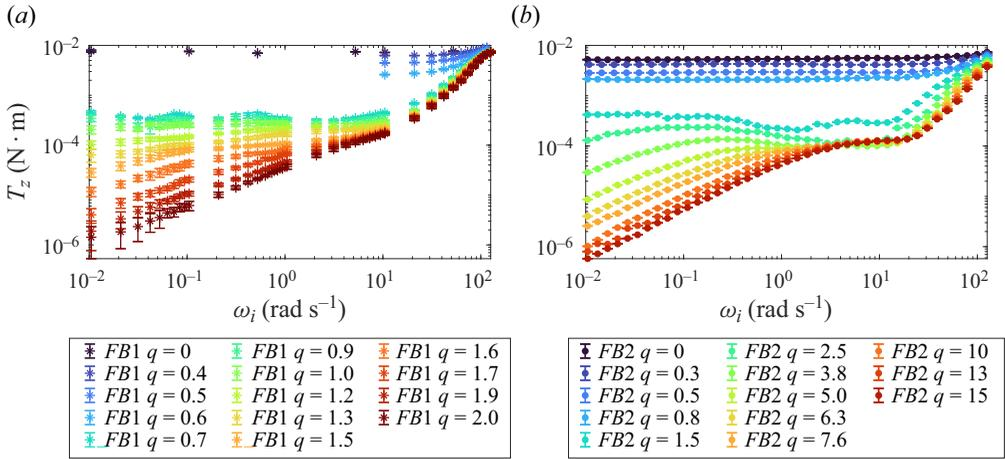
Figure 4. Measured torque as a function of angular velocity and fluidization rate for the *FB1* (a) and *FB2* (b) experiments. At different values of  $q$  and  $\omega_i$ , the torque measurements show quasistatic or viscous stress behaviour. Both *FB1* and *FB2* exhibit shear weakening near  $q \approx 1$  and at intermediate rotational speeds.
