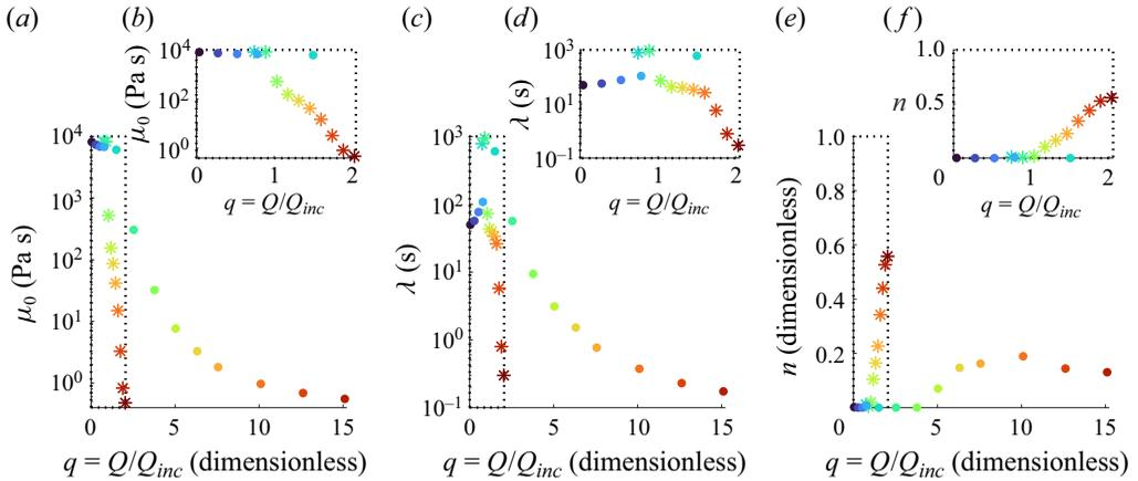
Figure 8. Fitted Carreau fluid parameters for the *FB* experiments as found in (5.8) against the normalized fluidization with (b), (d) and (f) showing  $q < 2$ . The initial viscosity,  $\mu_0$ , is shown in (a) and (b) and the relaxation time,  $\lambda$ , in (c) and (d). Panels (e) and (f) show the power index,  $n$ , which varies between 0 and 1 for shear-thinning Carreau fluids. The *FB2* experiments show a maximum with  $n = 0.19$ , whereas the *FB1* experiments increase up to  $n = 0.56$ .
