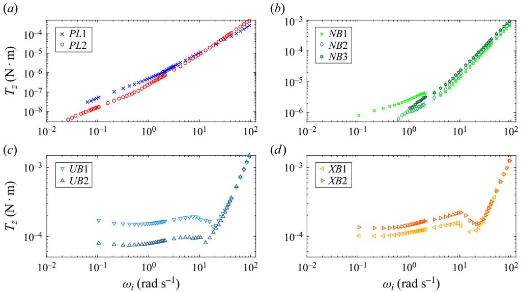
Figure 2. Measured torque against rotational speed for Newtonian liquids (*PL*, *a*), neutrally buoyant particle suspensions (*NB*, *b*), negatively buoyant particle suspensions (*UB*, *c*) and positively buoyant particle suspensions (*XB*, *d*).
