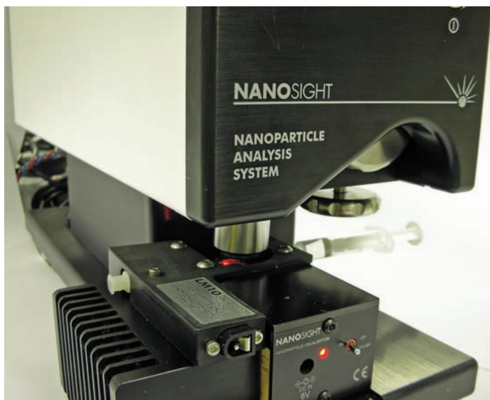
Figure 1: NanoSight LM20 nanoparticle characterization system with temperature stage attached for rigorous control.
