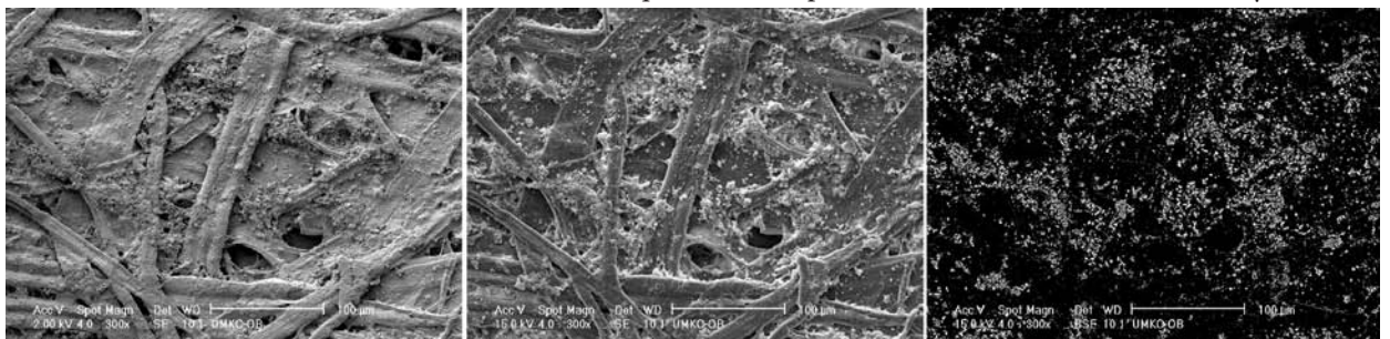
Figure 3. Writing paper. Secondary electrons at 2 kV (left), at 15 kV (center), and backscattered electrons (right).
