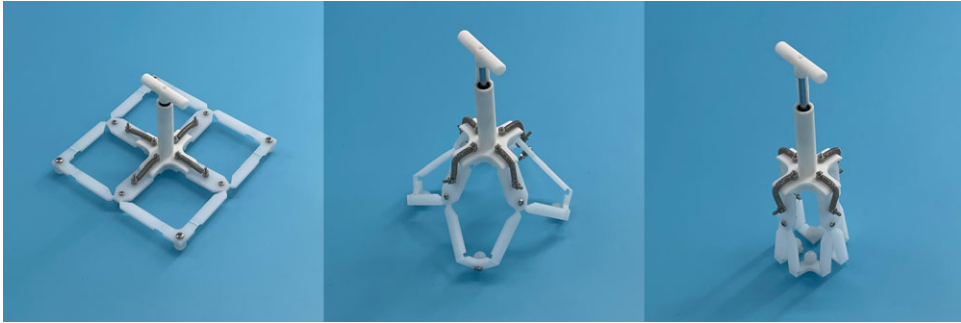
Figure 14. Grasping process of the compliant gripper.
