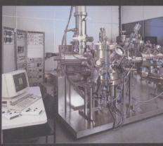
The versatile V80M thin film deposition system has up to 3" substrate capability. Its UHV growth chamber is fitted with three 40cc electron beam sources and three 40cc thermal effusion sources for flexibility in material choice. Provision is made for inlet of either neutral oxygen or an oxygen ion beam.
