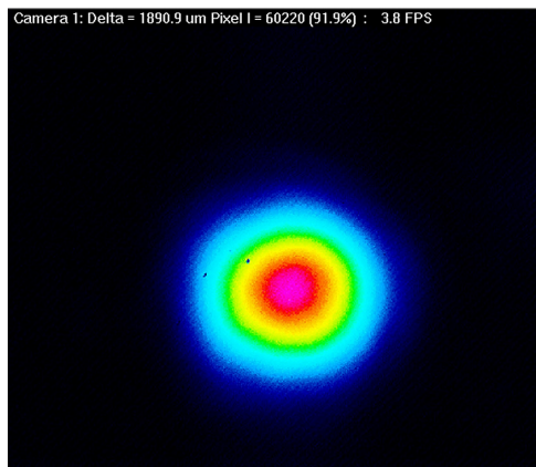
Figure 4. Beam profile of the oscillator output. As expected, the beam profile exiting from the oscillator is symmetric and has no intensity hotspot.
