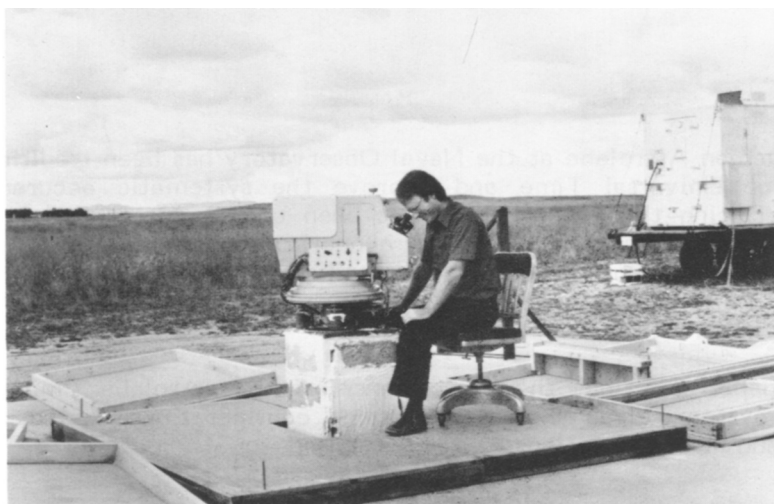
Figure 1. Astrolabe and shelter being installed at field site.
