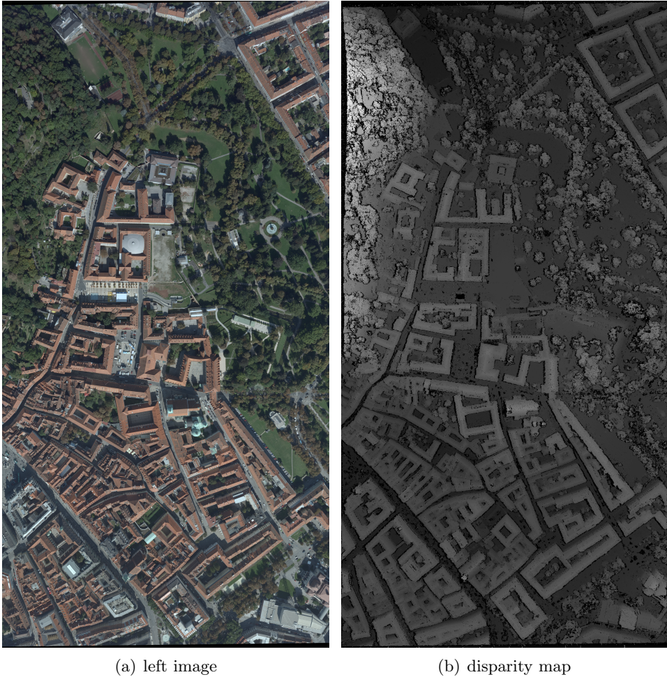
Figure 7.9. Computing a globally optimal solution of a large-scale stereo problem using the calibration method. (a) Left input image showing the region around the Freiheitsplatz in the city of Graz. (b) Computed disparity map, where the intensity is proportional to the height above the ground. Black pixels indicate occluded pixels that have been determined by a left-right consistency check.
