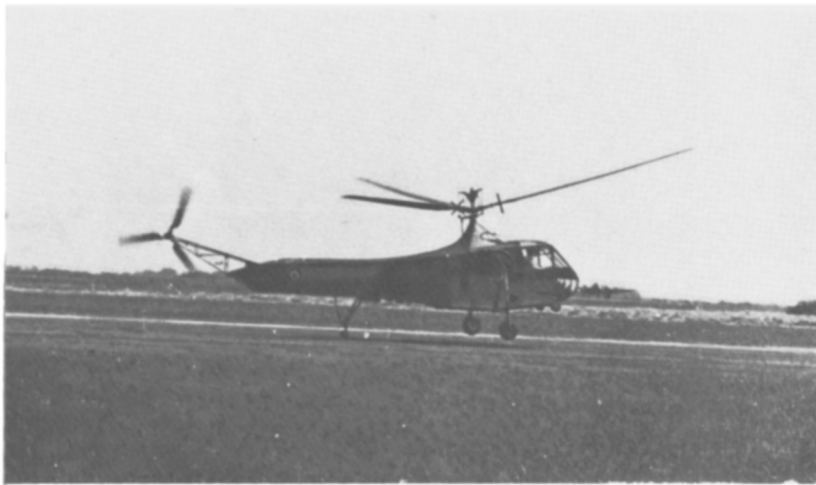
Fig 13 Engine-off landing attitude of Hoverfly I
