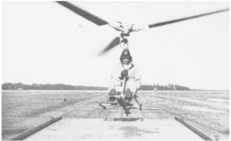
Fig 7 Kronfeld testing Fa 330 on short tow cable
