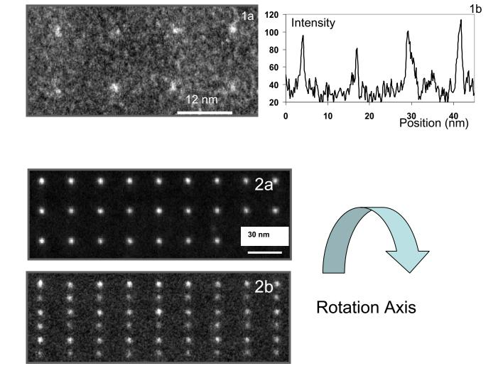
Figure 1: Z-contrast image (a) and associated line scan (b) show W dots with  $FWHM \sim 1 \text{ nm}$ .
