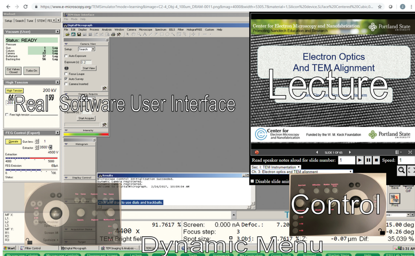
Figure 1: Image of the user interface showing the lecture content and microscope controls available. The OEMP offers high-fidelity online simulation of electron microscopes including lecture material and controls for interfacing with the virtual microscope.
