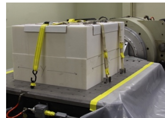
Figure 3. Foam-Mounted Flight Acceptance Vibration Test.
