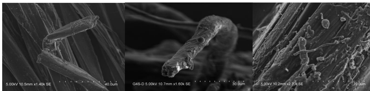
Figure 3. SEM micrographs of the historical fibres exhibiting fracture, roughened surface and biological colonization.
