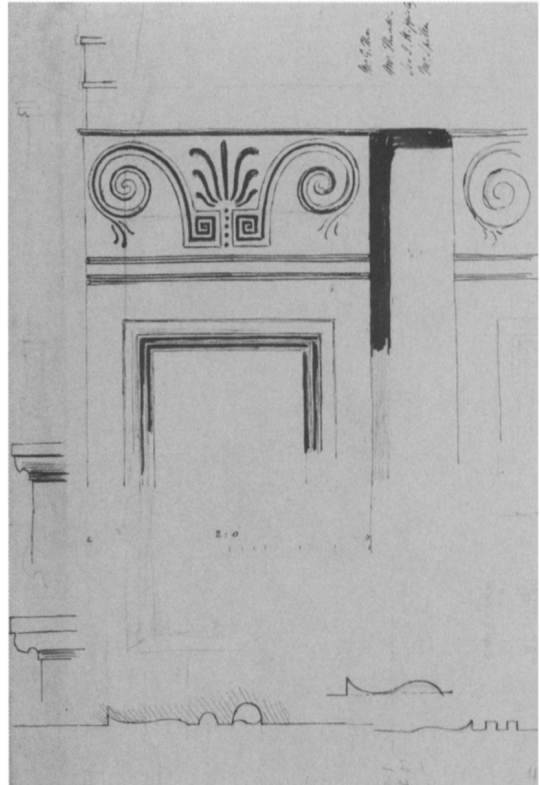
Fig. 20. Sketch design for a panelled pilaster with incised capital with volute, fret and anthemion motifs for the Consols Transfer House, Bank of England, by George Dance for Soane, c. 1799 (Soane Museum vol. 42/192)
