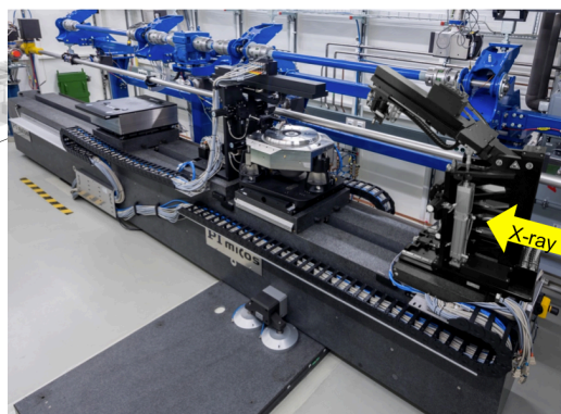
Figure 2. Photo of the experimental setup of the P05 nanotomography station. The 6.8 m long granite serves as an optical bench, equipped with 4 granite sliders. The blue structure in the back is a robot for moving the vacuum pipe in and out, switching between micro- and nanotomography stations EH1 and EH2.
