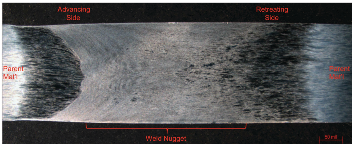
FIG. 2. Optical Micrograph of SR-FSW 2195 Al-Cu-Li Alloy
